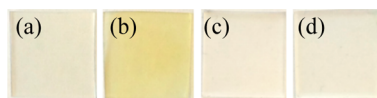
Figure 2. Polymer squares ( 1 \text{ cm}^2 ) of all samples tested for antimicrobial activity: (a) polyurethane control; (b) Cu-encapsulated polyurethane; (c) silicone control; (d) Cu-encapsulated silicone.
